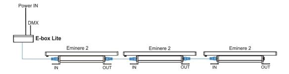
Number of connected Emineres to one E-box output depends on a cable length, power voltage, type of Eminere and E-box.
