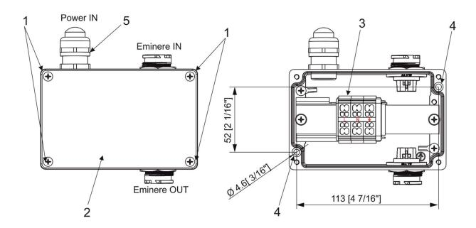
The Cable gland M20x1.5 for Power IN (5) is intended for a cable of a diameter of 7-13mm. Remove the end cap from the cable gland before passing the cable.
