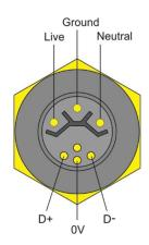
Output - panel connector (rear view - from side of soldering)
