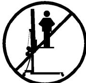
**3.1** - The TP-20 is a machine designed to elevate loads upwards in a vertical direction, It should NEVER be used as a platform to elevate people.
