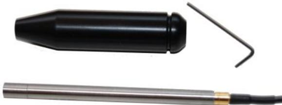
The bushing can be used together with the holding clamp or shockmount to attach the microphone to a regular microphone desk or floor stand. It is best not to clamp the microphone body but the SMB connector to avoid scratches or deformations on the microphone body. Attach the extension cable to the microphone and insert the microphone into the clamp. Use the Allen-key to fasten the screw slightly.
