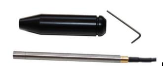
The bushing can be used together with the holding clamp or shockmount to attach the microphone to a regular microphone desk or floor stand. It is best not to clamp the microphone body but the SMB connector to avoid scratches or deformations on the microphone body. Attach the entension cable to the microphone and insert the microphone into the clamp. Use the Allen-key to fasten the screw slightly.
